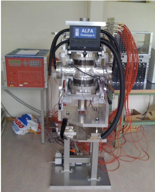
ALFA RP set-up before transport to H8 test beam zone.
