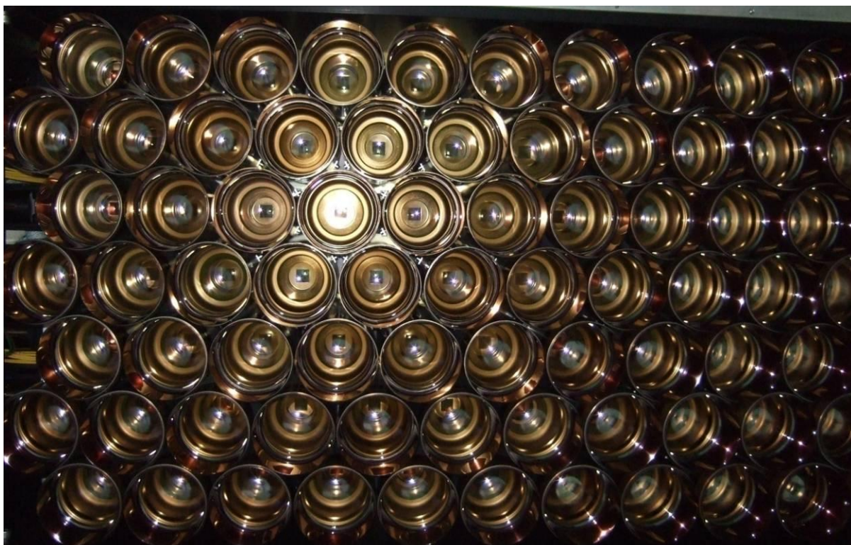
One HPD plane in the RICH1 detector (© R.Plackett from Imperial College London)
