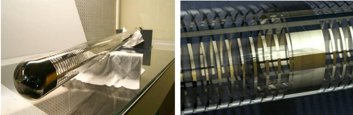
**Photos:** For the CLOUD Experiment, 2 quartz tubes have been partially coated with titanium to dissipate electrostatic charges on the surface.
