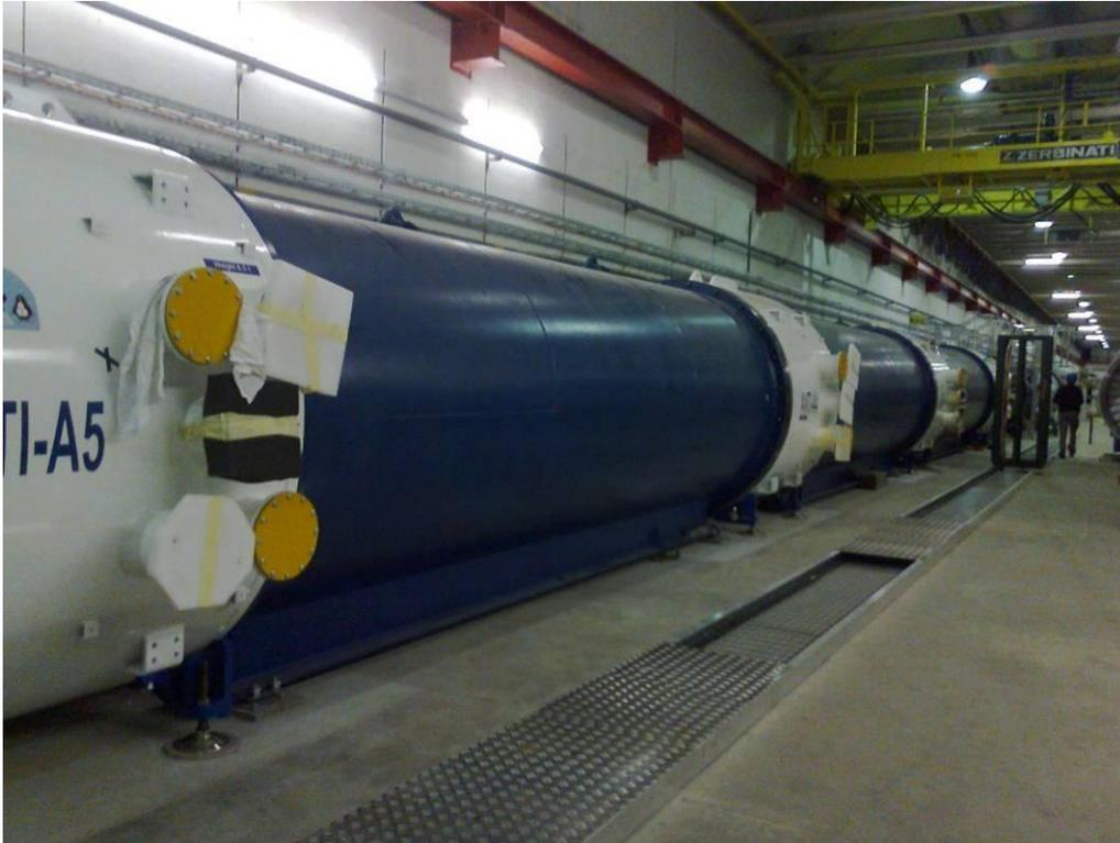
*Photo: Vacuum tanks and LAV detectors recently installed in TCC8.*
