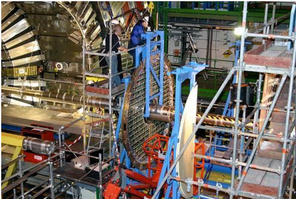
Figure 8 : CMS, installation of the pre-shower detector
