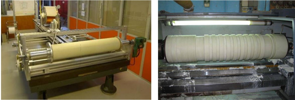
Figure 1 : Left hand side: The winding machine and the winding work shop in building 164. The winding support for the 1T solenoid is in position (the brown cylinder) and the spool of superconducting cable is ready (the orange cylinder partially covered by protection pasteboard). Right hand side: Machining of the winding support for the correction coils in a CNC lathe.
