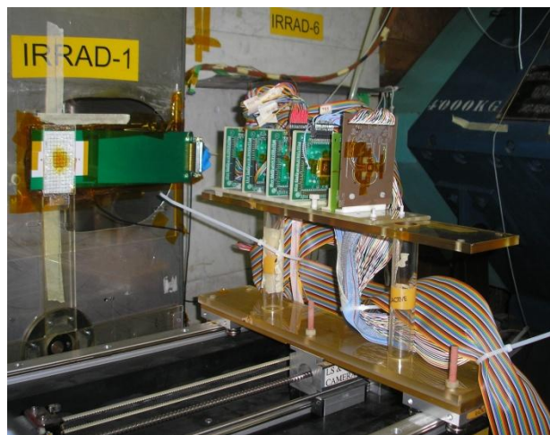
Irradiation test of prototype chips for the ATLAS Pixel upgrade (FEC4 in 130nm CMOS technology). In the background a new beam profile monitor is visible.
