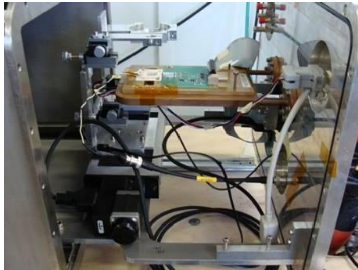
Setup to measure the Charge Collection Efficiency of silicon sensors, constructed by students and fellows of group. The setup can be operated at -20^{\circ}\text{C} .
