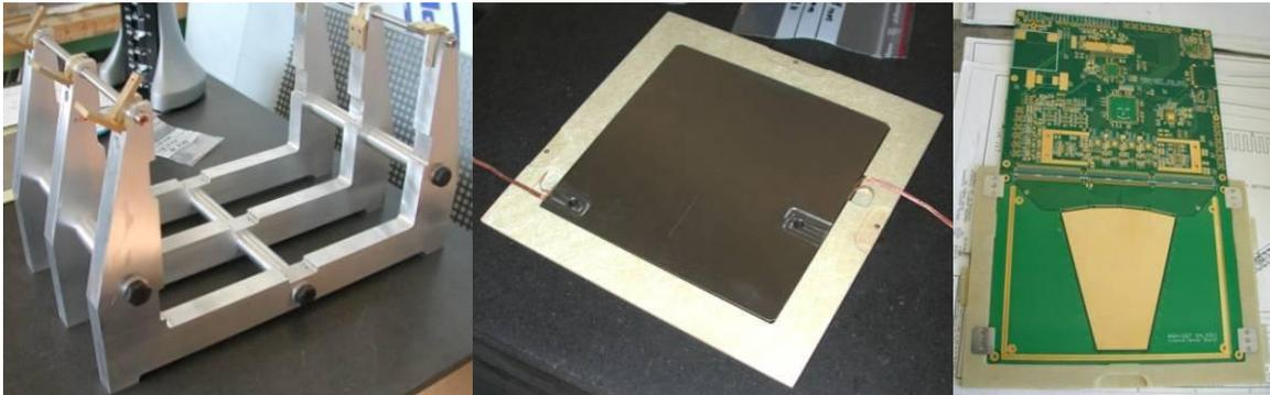
*Photos: The calorimeter frame, one tungsten plate in its permaglass holder, and a sensor in its holder.*
