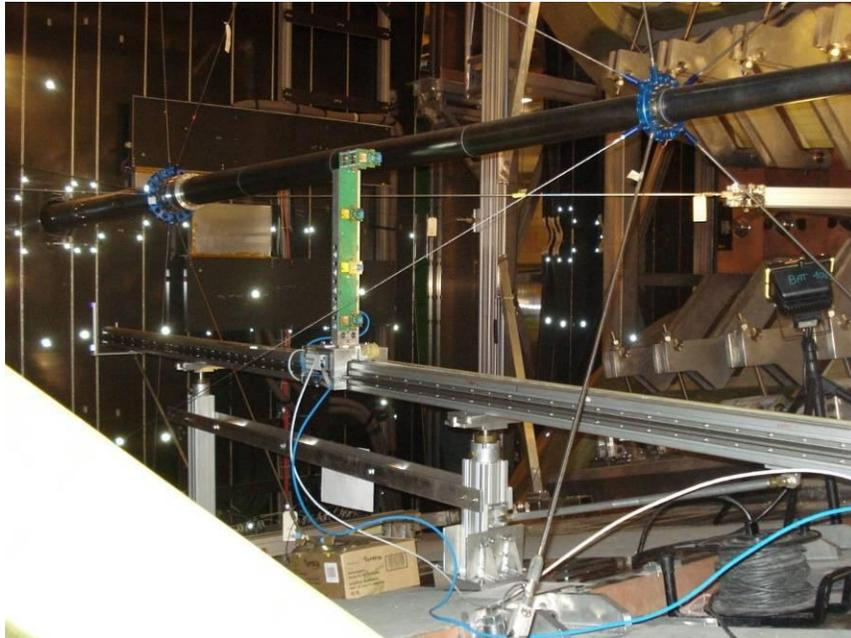
*Photo: LHCb magnetic field mapping near beam line with custom designed bench.*
