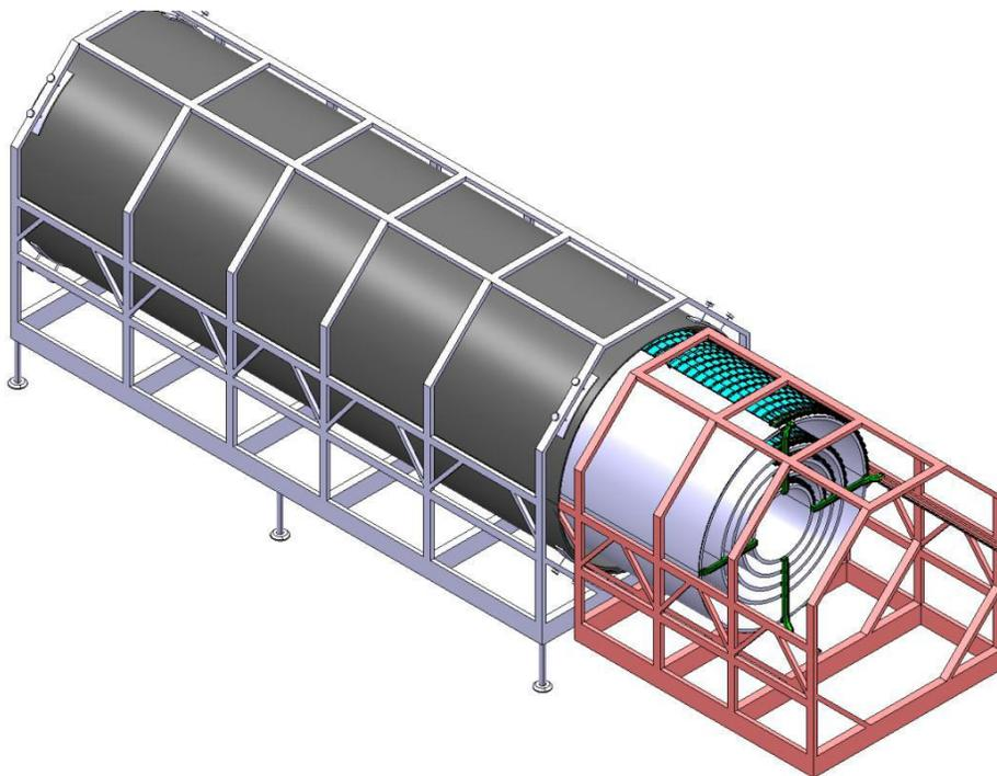
**3D CAD model image:** Surface assembly: insertion of the Barrel Strips into the tracker Outer Cylinder
