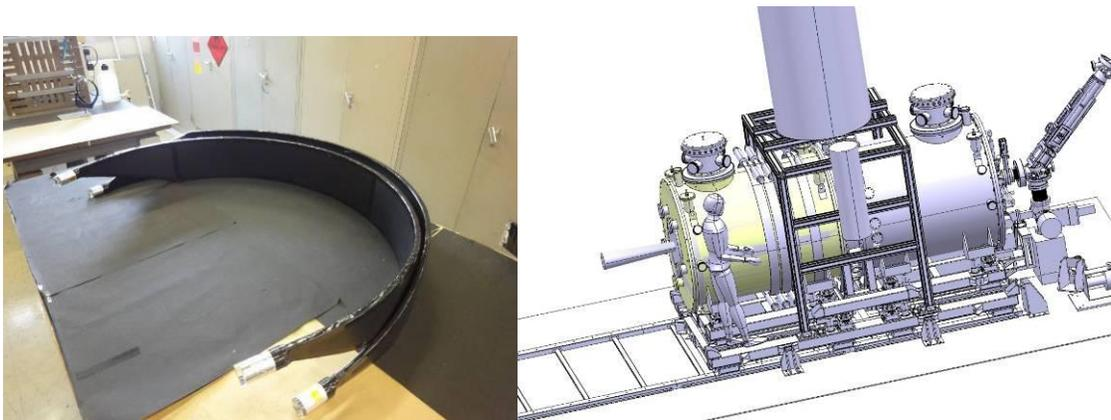
**Photo left:** Large semicircular scintillator bows for the AEGIS experiment. **CAD image right:** The Aegis experiment with the scintillators mounted..
