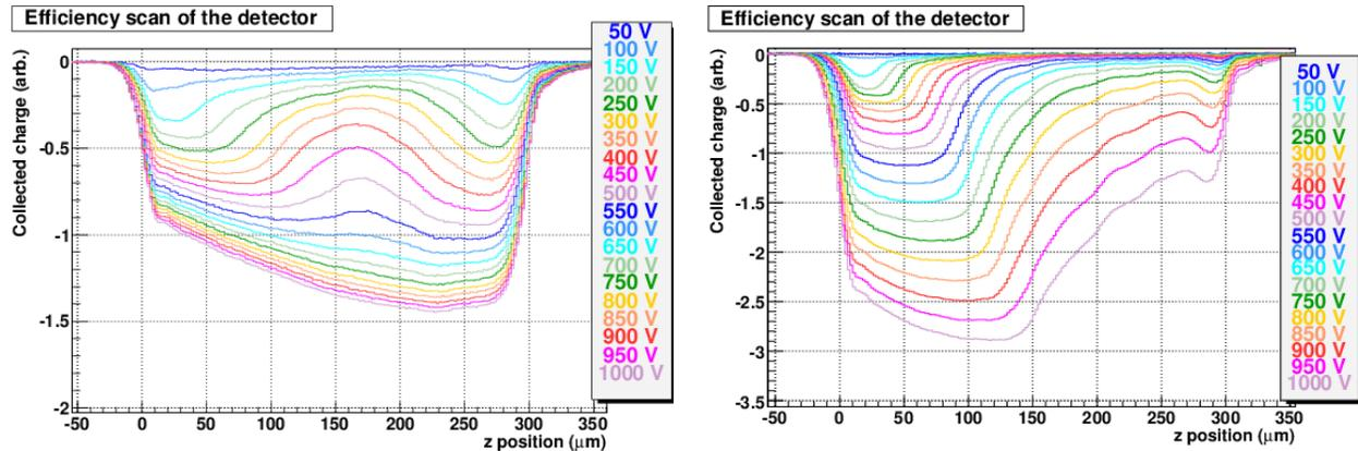
Efficiency depth profiles of an irradiated p-type silicon strip sensor directly after irradiation (left) and after an annealing of 10.000 minutes at 60°C. The front electrode corresponds to 0 μm and the 300 μm to the back electrode of the silicon sensor.
