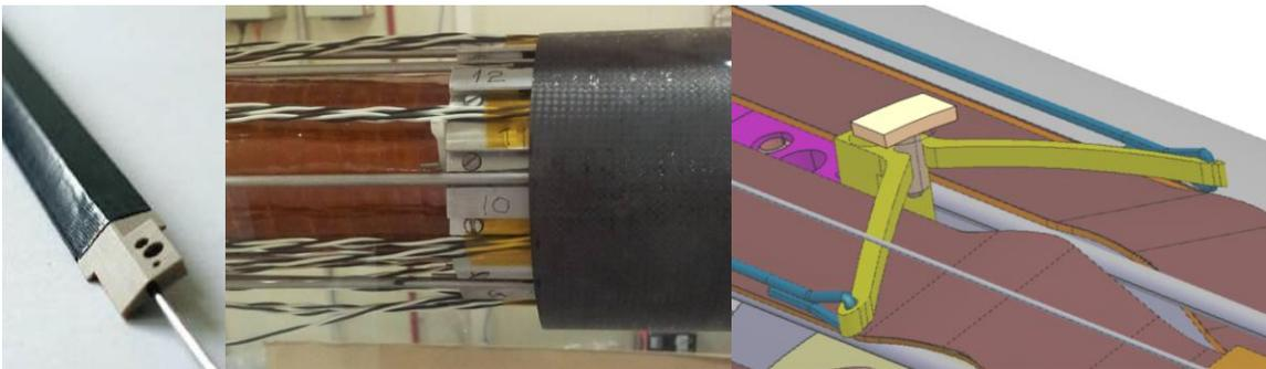
*Above pictures: Carbon fibre staves, the IBL thermal mock up assembly and the IBL integration concept.*
