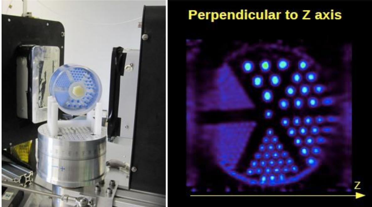
*Measurements at AAA with a FDG filled resolution phantom (produced in the DT workshop). Right hand side: Reconstructed image. The smallest resolved channels have a diameter of 1.6 mm and 3.2 mm between centres.*
