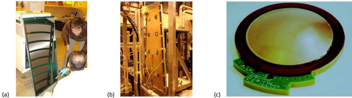
**Photos:** Large area MPGD detectors and detector components (a) Micromegas or ATLAS, (b) GEM for CMS and (c) spherical GEM for X-Ray diffraction application, developed within RD51 Collaboration with participation of PH-DT group.
