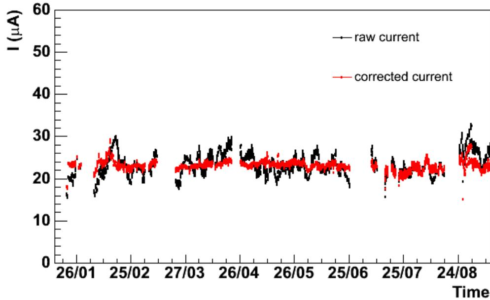
*The raw and corrected current drawn by the irradiated RPC's during the several months test period of the final optimized configuration of filters.*
